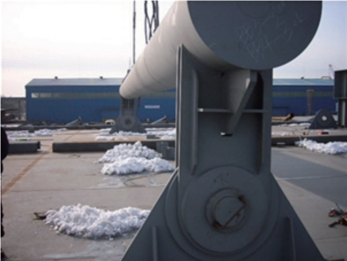
> LIFTING BEAM 체결 확인
